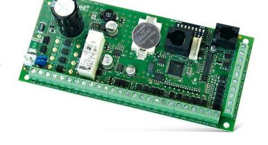
Configuration and some functions of ACCO–KP–PS might be different due to the system, which the controller is part of. Within the **ACCO** system the module is programmed by means of an LCD keypad or PC computer with **ACCO–SOFT–LT**
